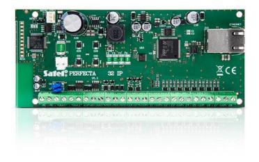
The system can be configured in two ways: from a computer with PERFECTA Soft program installed (locally – connection via RS-232 (TTL) port, remotely – using data transmission over Ethernet), as well as from a keypad, using key sequences in the service menu.
